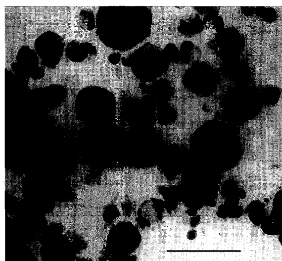
Fig. 5. Transmission electron micrograph of NiO/YSZ powder (bar = 100 nm).
